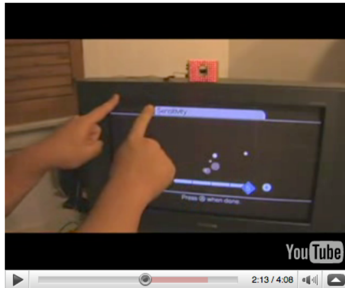
Figure 2.3: Finger tracking using an IR led array and reflective tape on fingers
